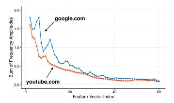
Fig. 3. Aggregate amplitudes corresponding to the first 60 bins computed from the power traces of google.com and youtube.com. (Corresponding time-domain traces are illustrated in Figure 2.) The *x* axis represents the index of each bin
