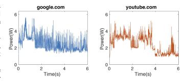
Fig. 2. Power traces collected during the first 6 seconds of automated webpage loading activity. The left and right panels show power traces collected while loading google.com, and youtube.com, respectively. The *x* axis shows time (in seconds) from the beginning of the webpage loading activity, and the *y* axis shows the power consumed by the smartphone.
