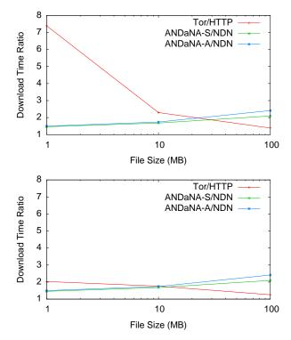
**Figure 2.** Comparison of 1, 10, and 100MB file download times over Tor, ANDāNA-S and ANDāNA-A with respect to respective baselines. Left: transfer time *and* circuit setup time. Right: transfer time only.
